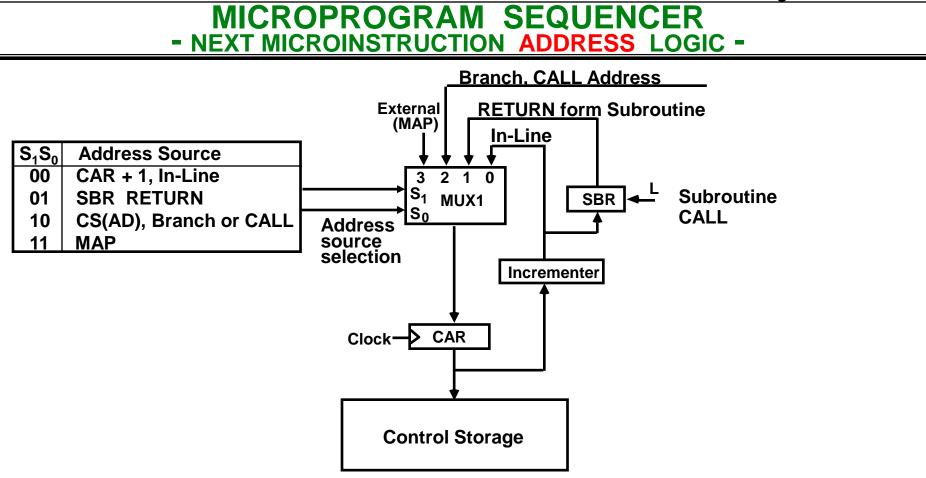
MUX-1 selects an address from one of four sources and routes it into a CAR
